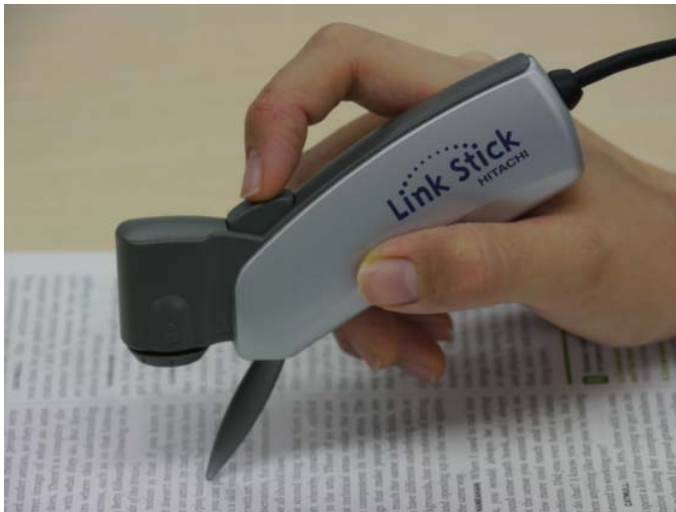
Fig. 2.19 The Hitachi LinkStick is a commercialized version of PaperLink. The pen has a built-in camera. From the camera image, a text pattern is extracted and acts as anchor for a hyperlink (photo courtesy of Toshifumi Arai)
