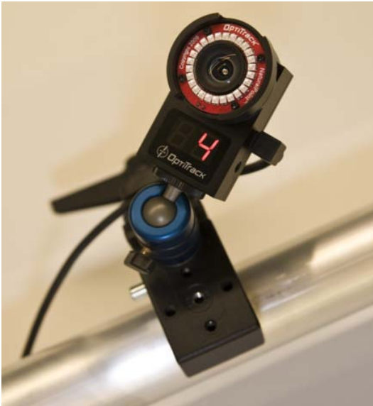
Fig. 2.3 An infrared camera of the OptiTrack high-speed motion capture system
